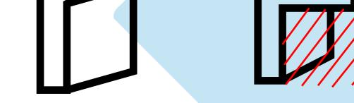
If two parts need to fit together loosely use a tolerance of 0.4 on every side of the model. Minimal: 0.2 mm tolerance Angles bigger than 45 degrees need support to print it properly. Try to make your angles 45 degrees and smaller to prevent printing support.
